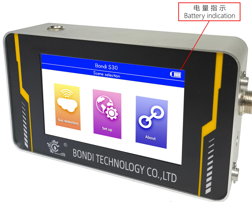
Figure 4.8 The work interface shows the battery level
