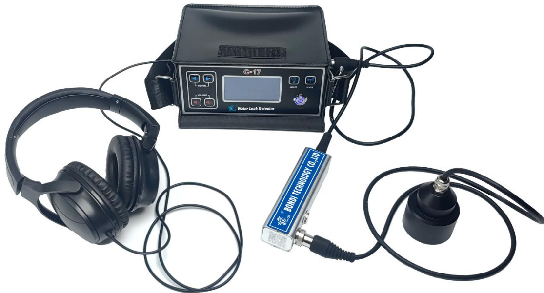
Figure 3.1 C-17 Installation and connection of pipeline leakage detector
