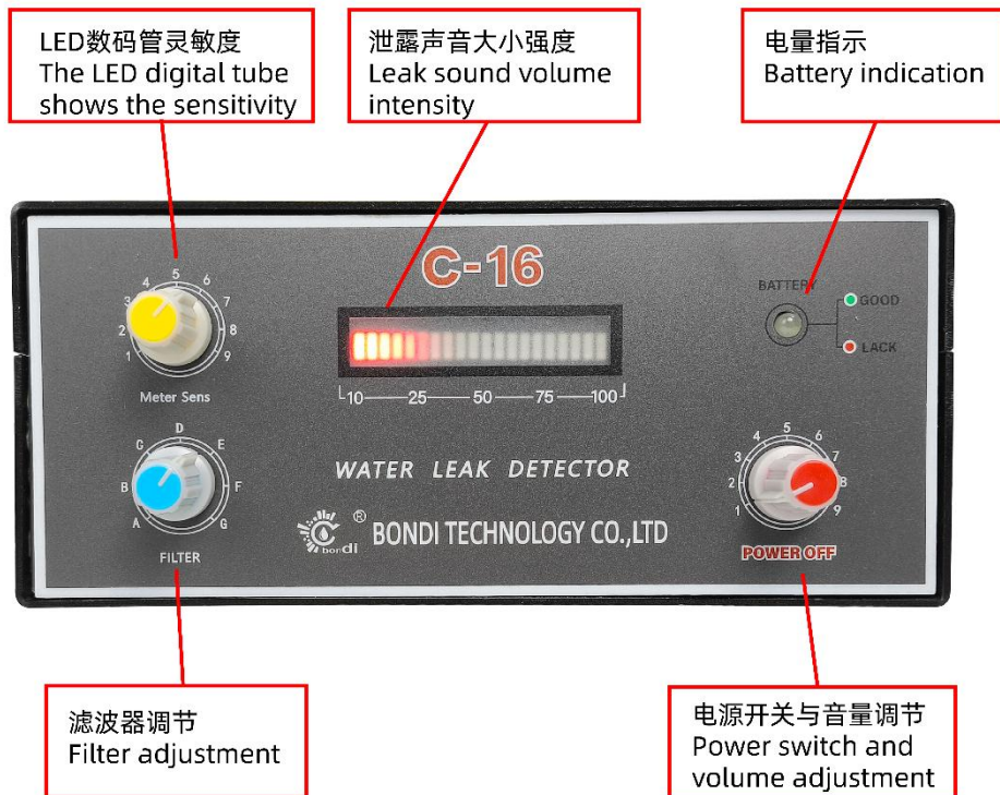
Figure 2.3 Operation interface
